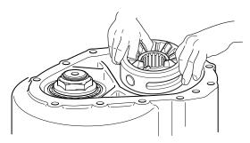
5. Install the helical side gear so that the clutch teeth are facing upward in the carrier.
