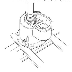
14. With 5 tons of force on the press, you should be able to feel a small amount of drag from the bearing as you rotate the carrier. If the carrier turns with no drag at all, the pinion spacer thickness should be decreased by using a thinner spacer. If the carrier is hard to turn, the spacer thickness must be increased.
