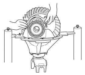
8. Use Dana's wheel diff. bearing adjustment tool (part number 513061) to back off the threaded cups and remove.
