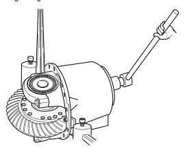
21. When contact pattern is correct. Use a punch with a round head to stake the threaded bearing cups in place. Stake the outer edge of the bearing adjustment ring into the machined slots in the carrier bearing bore on both sides. Must be staked at two locations. Rotate cup if necessary to provide surfaces for staking.
