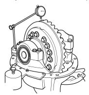
16. Check the ring gear tooth pattern. Paint 5 or 6 ring gear teeth 180 degrees apart on the ring gear.
