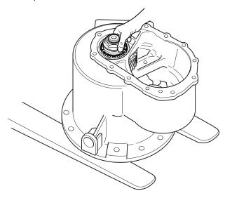
16. Run the nut down with an impact gun. The pinion should still have the same slight drag that was obtained in the press.
