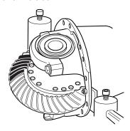
18. Make a sling out of a strap and position around the plain half of the wheel differential.
