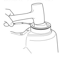
25. If a pilot bearing web is used, lineup the web to the locating sleeves and tap in place with a rubber mallet.
