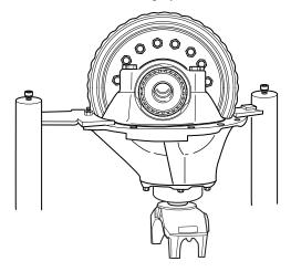
**Note:** For easier disassembly, loosen but do not remove the pinion nut.
