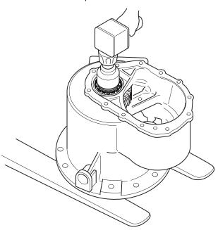
17. Secure the carrier in a head stand, rotate carrier so the pinion nut can be torqued.
