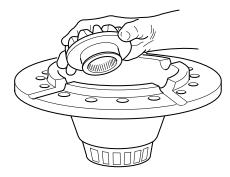
4. Assemble the side pinions onto the wheel differential spider. Apply a thin coat of oil to the mating surfaces of the side pinion and differential spider. Install the wheel differential nest on top of the side gear.
