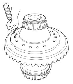
9. Install the ring gear capscrews.
