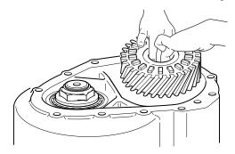
11. Remove the inter-axle differential assembly.
