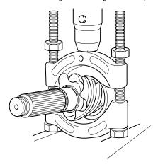
b. Mount the puller horizontally to press the bearing from the pinion.
