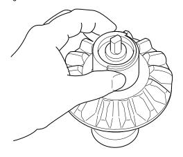
2. Install the pump locking dowel pin into the hole in the output side gear hub. Make sure the pin is lined up with the machined slot in the pump body.
