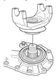
20. Install input shaft flanged nut and torque to the proper specifications. See Torque Chart.
