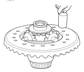
8. Install the flange half of the case. Align the capscrew holes.
