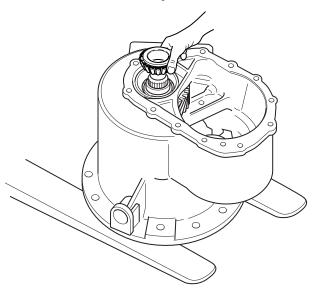
10. Install a pinion nut finger tight. This will hold the pinion in place while it is positioned into the press.
