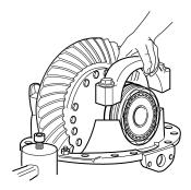
12. Use an impact gun to snug all carrier cap fasteners.
