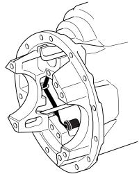
4. Fully press the manifold assembly into position.
