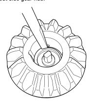
3. Remove pump from the output side gear.
