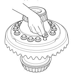
10. Tighten the ring gear capscrews with an impact gun and then use a torque wrench to torque to the proper specifications. See the Torque Chart.
