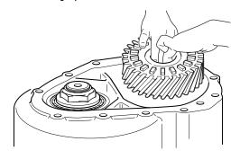
6. Install helical side gear thrust washer.
