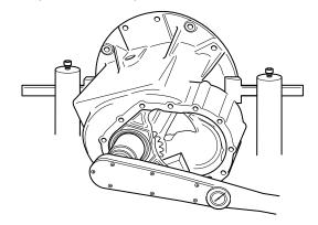
**TIP:** If you are unable to torque the yoke nut correctly, try torquing the nut with the truck wheels on the ground and with the axle shafts installed.
