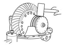
With a dial indicator, check the ring and pinion backlash. Set the backlash from 0.010" to 0.012". This will give you room to adjust the contact pattern, if necessary.
