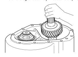
12. Assemble the sliding clutch, shift fork and fork spring to the input shaft and install assembly into carrier. Make sure that the shift fork rod is piloted in the carrier bore.
