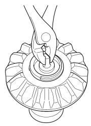
4. Remove the output side gear bearing cup from the carrier with the proper bearing puller tool.
