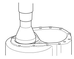
**Note:** If a press is not available, use a sleeve or bearing driver and a hammer to install the cups.
