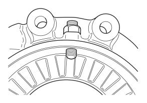
14. Input cage is threaded into the PDU cover, use the proper tool to remove the cage from the cover.
