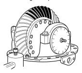
17. With the carrier mounted in a head stand, roll the carrier on its side.
