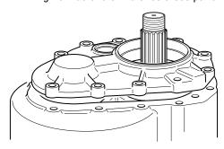
15. Install input shaft bearing adjuster, adjust inward until snug against the bearing cone.
