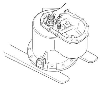
9. Install the outer bearing cone.
