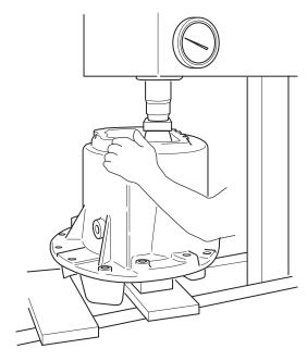
15. Remove the carrier from the press and reinstall the pinion nut.
