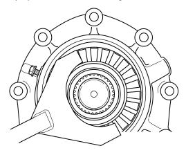
15. Use a suitable bearing puller to replace the input bearing cup.
