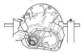
**Note:** Always use a new nut and coat threads with Loctite 277 if not pre-coated.
