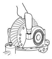
13. Recheck the backlash. For new gearing, the backlash should be between 0.008" and 0.018" (0.20 and 0.46 mm).
