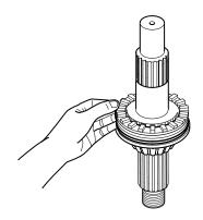
10. If removed, press the new input bearing cone in place until seated using the proper press sleeve or bearing installer.
