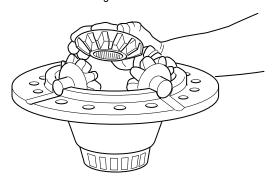
6. Install the ring gear. Align the capscrew holes.
