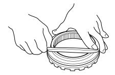
9. Install the sliding clutch so that the teeth are facing up.
