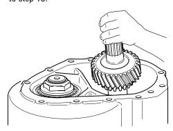
Remove the input shaft, sliding clutch, shift fork and spring as an assembly.
