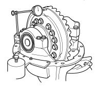
15. Measure the ring gear total backface runout. Indicator reading should not exceed 0.010" (0.25 mm).
