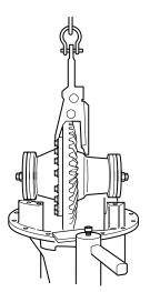
**Note:** There are two ways to make sure that the threaded cups are seated properly. If there is a misalignment, reinstall the differential assembly at a slightly different angle.
