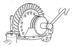
6. Turn the plain half adjuster ring until there is zero preload on the bearings. This is done by turning the adjuster plate clockwise until you feel the threaded cup gain resistance. The threaded bearing cup should only be slightly snugged to achieve a zero preload condition.
