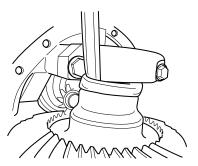
19. Connect the end of the strap to a hoist and apply pressure to the sling.
