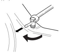
Plastic only: Tighten until one thread is showing.
