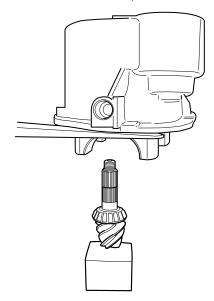
7. To align the splines of the helical gear to the pinion, use a old pinion nut with a metal ring welded to the top, thread onto the pinion. Then lift the pinion while aligning the two splined surfaces.
