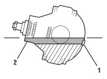
1 - Oil Filler Hole 2 - Lost Oil Capacity
