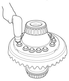
2. Remove the flange half differential case and bearing assembly. Use a screwdriver at the spider arm machined slots of the case to loosen the flange from the ring gear.
