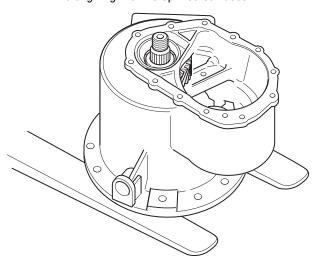
8. Install the pinion spacer.
