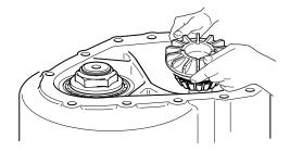
13. To replace the input bearing cup, back off the bearing cage locking fastener or jam nut and stud.
