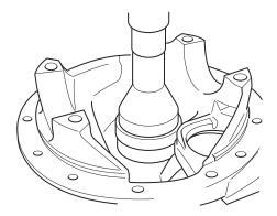
c. If replacement of the output shaft side gear bearing cup is necessary, use either of the following methods:
