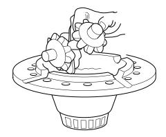
5. Install the flange half side gear. Apply a thin coat of oil to the mating surfaces.
