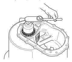
21. Once the proper rolling torque is achieved, use a punch with a round head to stake the nut collar into the slot in the pinion.
