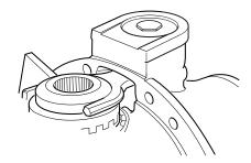
2. Remove the threaded cylinder cap.
