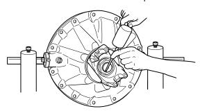
4. To de-stake the nut, use a chisel or drift with a round tip. The flange of the nut must be pushed far enough outward so that the staked area will not interfere with the pinion threads when the nut is removed. See diagram on next page.
