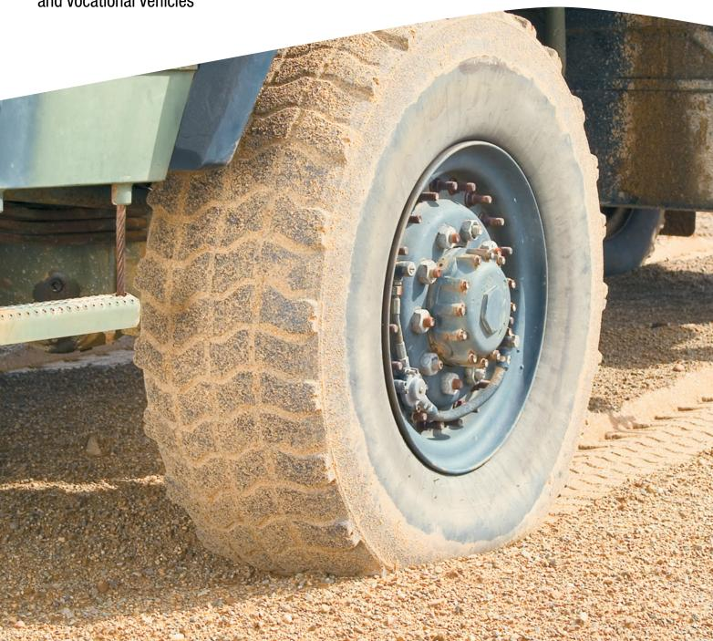
With the press of a button from inside the cab, Spicer® CTIS maximizes vehicle mobility by adjusting tire pressure to provide the optimum footprint on any terrain. Whether in the field or at a construction site, Spicer® CTIS promotes confidence on soft, sandy soil and other unpaved surfaces.
